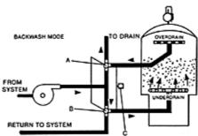
Five percent of 1200 gpm is 60 gpm, which requires a 24-inch filter with a flow rate of 63 gpm.
